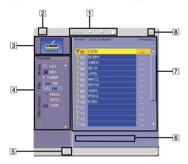
To view the TUNER window, click the TUNER icon in the Tool bar (page 7). Use this window to operate the tuner (page 77).
